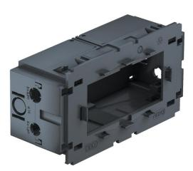
Front locking double accessory mounting box for Modul 45® system, with folding, and also removable, base for time-saving cable connection, with feed openings for cable diameters of up to 14 mm.
