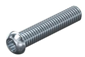
Flat head screw with TX 30, according to ISO 7380-1, suitable for fastening cable routes on brackets as well as for the mounting of barrier strips. The rounded head shape provides optimum cable protection. The Torx drive offers optimum force transmission in the screw movement.
