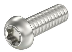
Flat head screw with TX 30, according to ISO 7380-1, suitable for fastening cable routes on brackets as well as for the mounting of barrier strips. The rounded head shape provides optimum cable protection. The Torx drive offers optimum force transmission in the screw movement.
