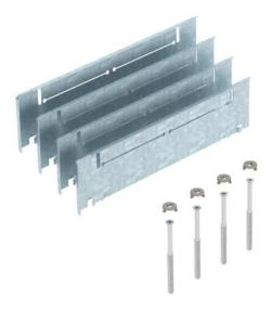
Height compensation set for underfloor boxes UZD250-3 and UGD250-3 with a construction height of 70 to 125 mm for construction stacking of the UZD/UGD to a height of 115-170 mm, consisting of four fall plates, four height adjustment screws and four rotary locks.
