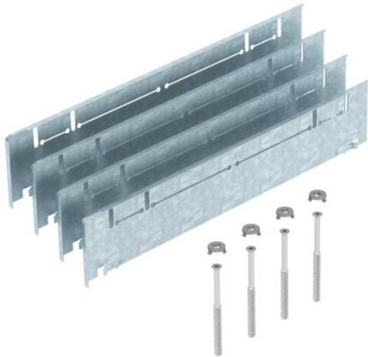
Height compensation set for underfloor boxes UZD350-3 with a construction height of 70 to 125 mm, consisting of four fall plates, four height adjustment screws and four rotary locks.
