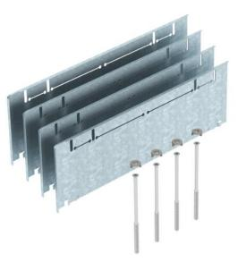
Height compensation set for underfloor boxes UZD350-3 with a construction height of 70 to 125 mm, consisting of four fall plates, four height adjustment screws and four rotary locks.
