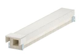
Fire protection duct made from water and frost-proof fibreglass light concrete of building material class A1 according to EN 13501-1 for fireproof laying of cables in rescue and emergency routes, and for the maintenance of electrical functionality of safety-relevant systems. Classification I90 as I duct according to DIN 4102 Part 11 and classification E30 as E duct according to DIN 4102 Part 12.
