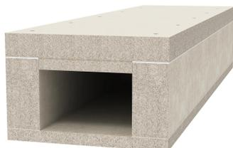
Fire protection duct made from water and frost-proof fibreglass light concrete of building material class A1 according to EN 13501-1 for fireproof laying of cables in rescue and emergency routes, and for the maintenance of electrical functionality of safety-relevant systems. Classification I120 as I duct according to DIN 4102 Part 11 and classification E90 as E duct according to DIN 4102 Part 12.
