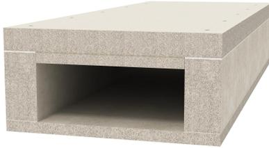
Fire protection duct made from water and frost-proof fibreglass light concrete of building material class A1 according to EN 13501-1 for fireproof laying of cables in rescue and emergency routes, and for the maintenance of electrical functionality of safety-relevant systems. Classification I120 as I duct according to DIN 4102 Part 11 and classification E90 as E duct according to DIN 4102 Part 12.
