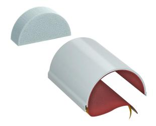
Internally coated half shell, the inner space of which can be fully assigned with cables and electrical installation pipes. For interior application. CE-labelled, European approved construction product according to ETA-13/0904 and German general type approval. Fire resistance up to 120 minutes.
