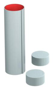
Internally coated pipe shells with click lock. The inner space can be fitted with cables and electrical installation pipes completely. For interior application. CE-labelled, European approved construction product according to ETA-13/0904 and German general type approval. Fire resistance up to 120 minutes.
