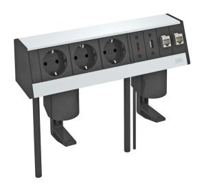
Deskbox with connection cable, cable outlet at the bottom of the profile with two fastening clamps for tabletop thicknesses of 8 to 40 mm.
