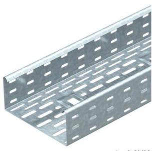
DKS 85 = perforated cable tray system with 85 mm side height. Permeable cable tray system to VdS guideline 2092 with 30% hole surface for use under sprinkler systems. Bottom penetration from width 200 mm.
