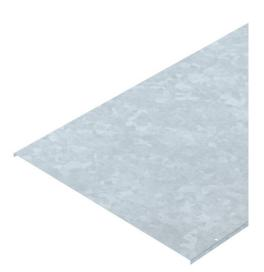
Unperforated cover for cable trays and cable ladders in indoor and outdoor areas, for the protection of the cables against damage and dirt. Fastening with cover clamp. When the cover is used under the impact of wind, suction or pressure, additional securing measures must be carried out.
