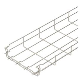
Mesh cable tray with shaped connector of side height 55 mm. No additional connection components are required for the mesh cable tray, it is simply interlocked. The grid width is  $50 \times 100 \text{ mm}$  (exception: GRM  $55/50 = 20 \times 100 \text{ mm}$ ).
