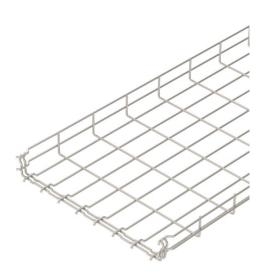
Mesh cable tray with shaped connector of side height 55 mm. No additional connection components are required for the mesh cable tray, it is simply interlocked. The grid width is  $50 \times 100 \text{ mm}$  (exception: GRM  $55/50 = 20 \times 100 \text{ mm}$ ).
