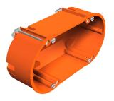
Double device socket, for two service outlets or one double service outlet, with four device screws. Dimensions to DIN 49073-1, for plate thickness 7–35 mm. Standard combination spacing 71 mm,
