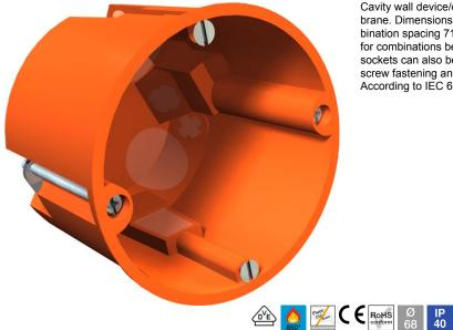
Cavity wall device/connection socket, wind-tight version through soft entry membrane. Dimensions to DIN 49073-1, for plate thickness 7–35 mm. Standard combination spacing 71 mm, option for continuous wiring using connection supports for combinations between device sockets and device connection sockets. Device sockets can also be used as connection sockets to VDE 0606-1 with double screw fastening and screw-on cover, protection rating IP40. According to IEC 60670-1, IEC 60670-22 and DIN 49073-1.
