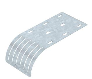
Drop-out plate for mesh cable trays. The exit plate allows compliance with specific bend radii, thus preventing possible cable breaks. Can be mounted in a lengthwise direction and at the side, can also be arranged next to each other for greater widths.
