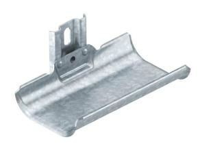
Cable support brackets for quick and easy routing of cables in areas where common cable support systems cannot be installed due to lack of space. The cable support brackets possess a large load-bearing surface as well as rounded outer edges to protect the cables.
