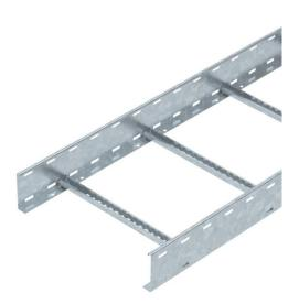
Cable ladder with 110 mm side height with welded C30 profile rungs which are open in an upwards direction. Rolled side rail for reinforcement and as edge protection. Fastening to the bracket takes place using clamps, type LKS 40. The slot dimension of the frame is 16.5 mm and the appropriate clamp clip is type 2056.
