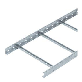
Cable ladder with a 60 mm side height with welded C30 profile rungs which are open in an upwards direction. Rolled side rail for reinforcement and as edge protection. Fastening to the bracket takes place using hold-down clamps, type LKS 40. The slot dimension of the rung is 16.5 mm and the appropriate clamp clip is type 2056.
