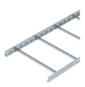
Cable ladder with a 60 mm side height with welded C30 profile rungs which are open in an upwards direction. Rolled side rail for reinforcement and as edge protection. Fastening to the bracket takes place using hold-down clamps, type LKS 40. The slot dimension of the rung is 16.5 mm and the appropriate clamp clip is type 2056.
