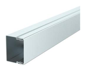
Duct cover and base with base perforation. Equipotential bonding is guaranteed between the cover and the base without any additional aids. The LKM cable duct, type LKM 20030, has been tested for the maintenance of electrical function as a routing system according to DIN 4102 Part 12. Please note the cable types tested in the BSS fire protection systems division!
