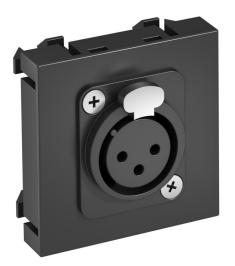
Multimedia support with one XLR connection socket, straight cable outlet, without labelling panel, 3-pin XLR socket with soldered connection. Support plate with locking fastening, suitable for horizontal and vertical installation in the system environment.
