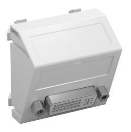
Multimedia support with one DVI-D connection socket, slanting cable outlet, with labelling panel, DVI-D socket with screw connection. Support plate with locking fastening, suitable for horizontal and vertical installation in the system environment
