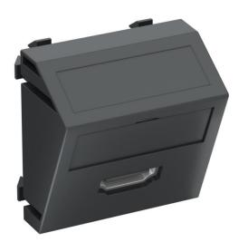
Multimedia support with one HDMI connection socket, slanting cable outlet, with labelling panel, HDMI socket with screw connection. Support plate with locking fastening, suitable for horizontal and vertical installation in the system environment.
