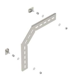
$90^\circ$  installation profile, vertical, for C mesh cable tray and GR-Magic® mesh cable tray with a side height of 55 mm. Each with two clamps of type KS 23/35. Including connector, to create  $45^\circ$  bends.
