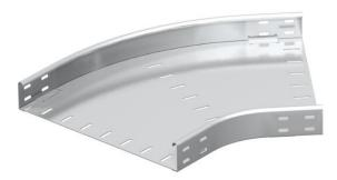
$45^\circ$  bend, horizontal and unperforated, for all cable tray types of 60 mm side height. Fitting, unperforated, in round design. The interior radius of the fitting is 150 mm. Fastening materials should be ordered separately.
