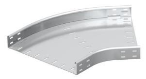
$45^\circ$  bend, horizontal and unperforated, for all cable tray types of 60 mm side height. Fitting, unperforated, in round design. The interior radius of the fitting is 150 mm. Fastening materials should be ordered separately.
