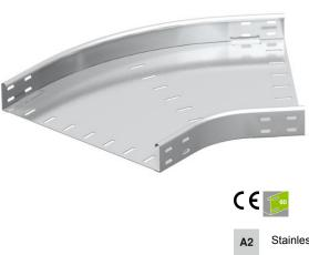
45° bend, horizontal and unperforated, for all cable tray types of 60 mm side height. Fitting, unperforated, in round design. The interior radius of the fitting is 150 mm. Fastening materials should be ordered separately.
