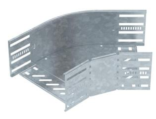
45° bend for the creation of a horizontal branch, fitting for lock and screw-on cable trays of side height 110 mm. Screwless mounting with double clamps or screw connection with FRS truss-head screws and M6 combination nuts. Can be used indoors and outdoors. Fastening material must be ordered separately.
