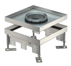
Heavy-duty square cassette for tube body of nominal size 9 for the installation of accessories in trunking systems, raised or cavity floors, in dry or wet-cleaned floors for indoor use. Load class 1 to 10 kN.
