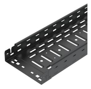
Cable tray with integrated quick-fastening system. Strip-galvanised surface, visible areas powder-coated in jet black (RAL 9005). Continuous side perforations of 7 x 20 mm for the installation of additional connection and mounting components. With 11 mm perforation in the base for direct threaded rod suspension. Usable length 3,000 mm.
