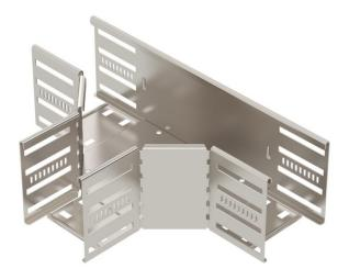
T piece for the creation of a horizontal branch, fitting for lock and screw-on cable trays of side height 110 mm. Screwless mounting with double clamps or screw connection with FRS truss-head screws and M6 combination nuts. Can be used indoors and outdoors. Fastening material must be ordered separately.
