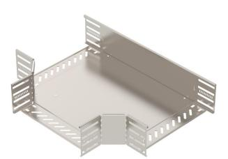
T piece for the creation of a horizontal branch, fitting for lock and screw-on cable trays of side height 110 mm. Screwless mounting with double clamps or screw connection with FRS truss-head screws and M6 combination nuts. Can be used indoors and outdoors. Fastening material must be ordered separately.
