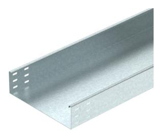
SKS 85 = Heavy-duty cable tray system, unperforated, with 85 mm side height. The cable tray has connector perforations on both sides. Straight connectors should be ordered in the appropriate quantity. Magnetic shield insulation without cover 20 dB, with cover 50 dB.
