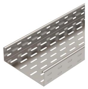
SKS 60 = heavy-duty cable tray system with 60 mm side height. The cable tray, type SKS, should also be used for maintenance of electrical function. For additional data, please refer to BSS fire protection systems. The cable tray is fastened to the bracket with bolts, type FRS M6 x 12.
