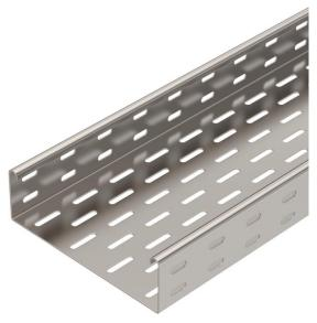
SKS 60 = Heavy-duty cable tray system with 60 mm side height. The cable tray, type SKS, should also be used for maintenance of electrical function. For additional data, please refer to BSS fire protection systems. The cable tray is fastened to the bracket with bolts, type FRS M6 x 12. Magnetic shield insulation without cover 20 dB, with cover 50 dB.
