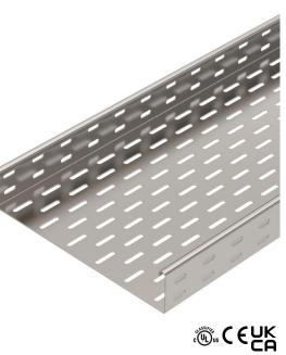
SKS 60 = Heavy-duty cable tray system with 60 mm side height. The cable tray, type SKS, should also be used for maintenance of electrical func-tion. For additional data, please refer to BSS fire protection systems. The cable tray is fastened to the bracket with bolts, type FRS M6 x 12. Magnetic shield insulation without cover 20 dB, with cover 50 dB.
