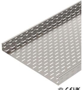
SKS 60 = heavy-duty cable tray system with 60 mm side height. The cable tray, type SKS, should also be used for maintenance of electrical function. For additional data, please refer to BSS fire protection systems. The cable tray is fastened to the bracket with bolts, type FRS M6 x 12.
