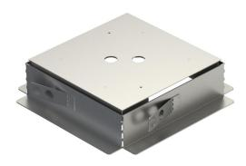
Lined body, suitable for polishing, for the direct and jointless installation of height-adjustable cassettes, nominal size 4, into surface-finished screeds/terrazzo floorings. The casing is laid floatingly onto underfloor boxes with mounting lids of nominal size 4, closing the gaps between underfloor box and cassette frame. The protection cover made from aluminium sheet is put into the cassette frame as a dummy before the screed work is done and can be polished over with the screed or terrazzo.
