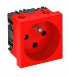
Socket with earthing pin, single  $0^\circ$ , encoded version, with increased touch protection, with screwless terminals, 2-pin, 16 A, 250 V $\sim$ , with connection terminals according to IEC 60884-1.
