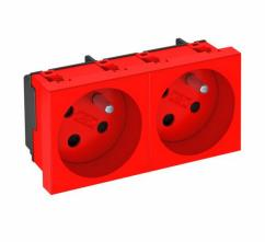
Socket with earthing pin Double 33°, encoded version, with increased touch protection, with screwless terminals, 2-pin, 16 A, 250 V $\sim$ , with connection terminals to IEC 60884-1. The socket can only be used in conjunction with an encoding pin, type CST-STD.
