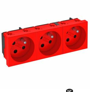
Socket with earthing pin Triple 33°, encoded version, with increased touch protection, with screwless terminals, 2-pin, 16 A, 250 V~, with connection terminals to IEC 60884-1. The socket can only be used in conjunction with an encoding pin, type CST-STD.
