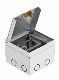
Square floor socket for use in dry-care cavity and screed floors in indoor areas. Installation housing with pre-marked insertion openings for pipes (M25). Cover adjustable to top edge of floor covering using four height-adjustment supports. The minimum installation depth is 95 mm, the height-adjustment range +20 mm.
