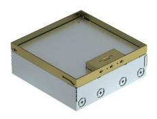
Square floor box for use in dry-cleaned cavity and screed floors in indoor areas. Installation housing with pre-marked insertion openings for pipes (M25). With three UT4 universal supports and two double sockets. Cover adjustable to top edge of floor covering using four height-adjustment supports. The minimum installation depth is 95 mm, the height-adjustment range + 30 mm.
