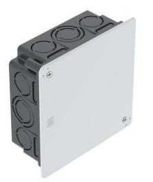
Flush-mounted connection box for clamping terminals, for use in masonry with an installation depth of at least 45 mm. With cover and cover screws (15 mm). Flat cover edge, roughened surface.
