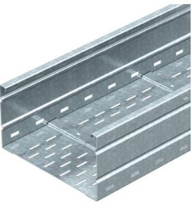
Wide span cable tray system, perforated, with a side height of 160 mm. Straight connectors of type WRV 160 should be ordered separately and in the appropriate quantity. Magnetic shield insulation without cover 20 dB, with cover 50 dB.
