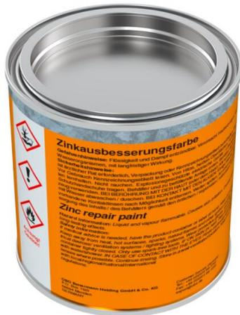
Zinc repair paint for blank areas on the hot galvanised steel parts, to eliminate grinding and welding damage on the galvanisation and to adapt ungalvanised small parts on galvanised structures.
